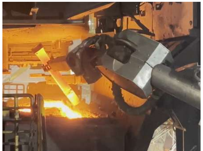
PolyCAST: Multitool robotic solution for caster operations
