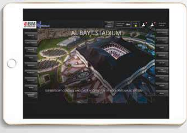
HMI for the management of Al-Bayt stadium's roof
